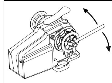
**⚠ Make sure the anchor windlass is not powered before carrying out manual interventions.**
