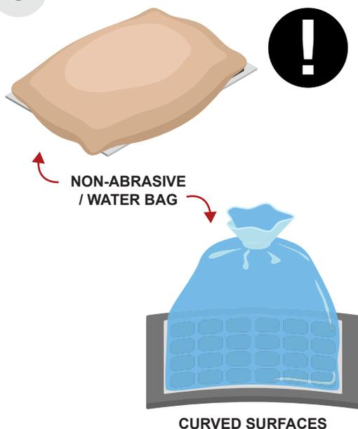
**EN** Use a non-abrasive weighted bag (e.g. sand/water bag) to achieve even and firm pressure while curing, ensuring no part of the panel lifts off the surface. Do this for flat but especially for slightly curved surfaces. Never use vacuum to shape the panel.
