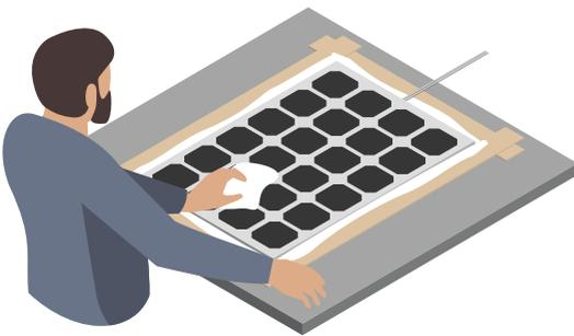
**EN** Start with one edge and carefully position and lower the panel on the surface, applying light and even pressure to press out any air underneath the panel.
