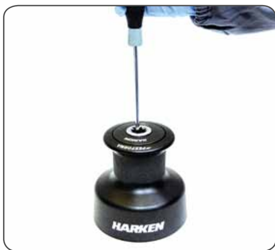
1. Unscrew the central screw (2Nm/18 in-lb)
