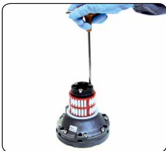
4. Completely unscrew the three screws n° 27
