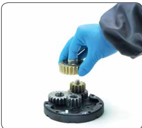
10. Remove the gearing n°7 and remove the pawls n°5. To facilitate the operation press the spring against the pawl with a blade.
