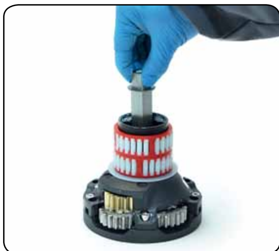
6. Slide out the central shaft n° 19
