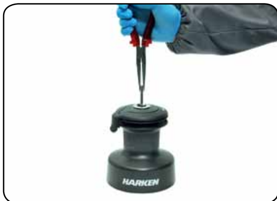
1. Pull out the disconnect rod n°28
