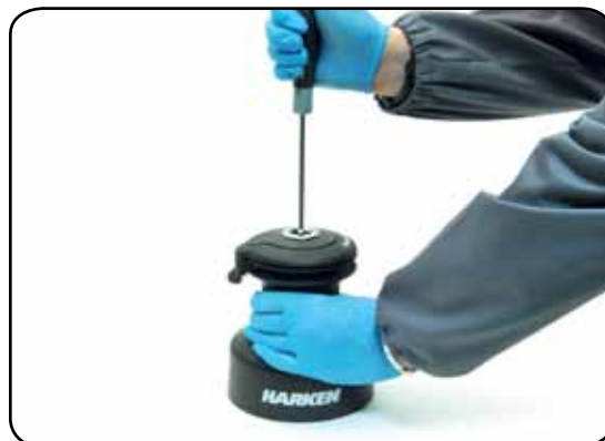
2. Unscrew the central screw ( \approx 2\text{Nm}/18\text{ in-lb} )
