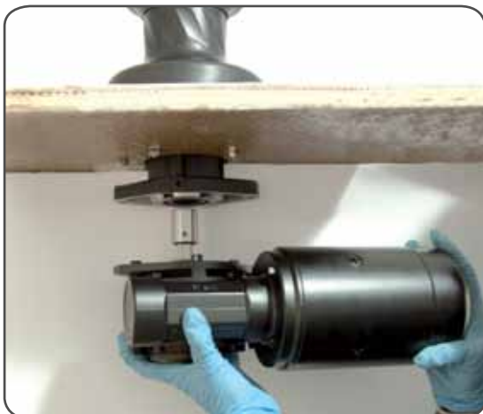
3. Position the reduction gear and motor
