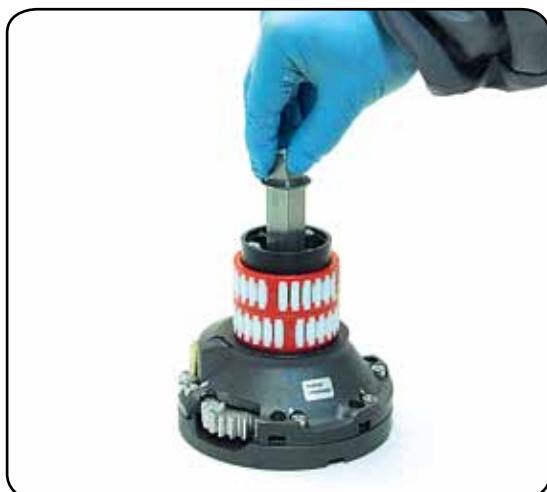
9. Slide out the central shaft n°18
