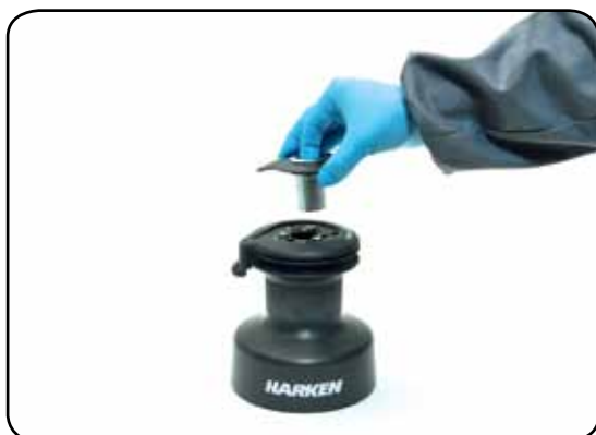
3. Slide off the assy socket n°26 and the cover n°27. Pay attention to the o-ring in the socket.
