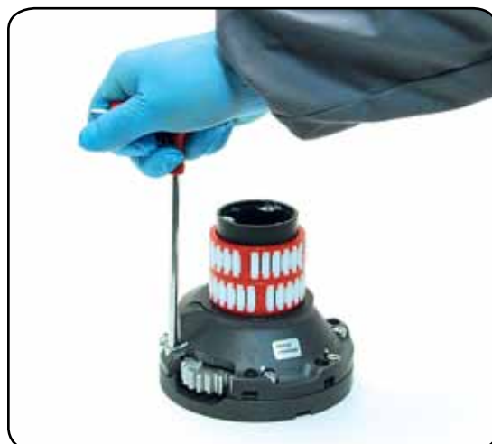
10. Unscrew the 6 hex screws n°15 ( \approx 8\text{Nm}/71\text{ in-lb} )
