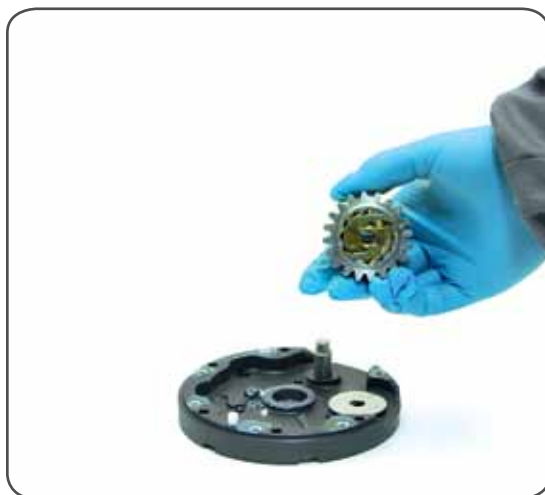
18. Remove the pawls n°4. To facilitate the operation press the spring against the pawl with a blade.
