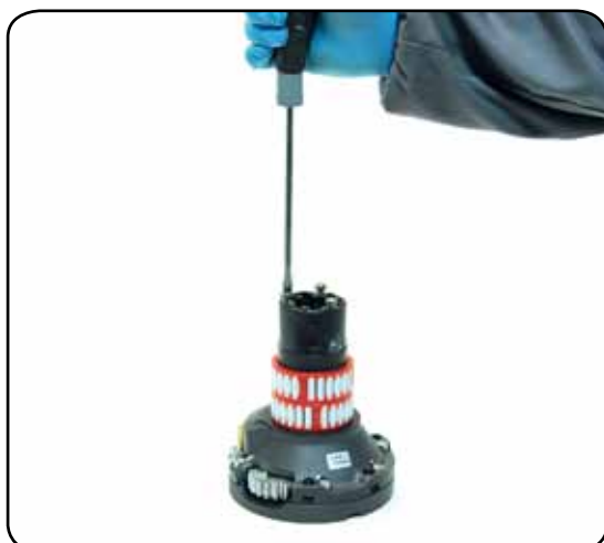
7. Completely unscrew the three screws n°25
